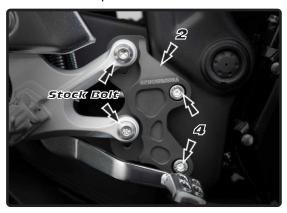
Install (No. 5) 13320-RSV-BKT, reservoir bracket using the stock bolt. Secure rear brake reservoir to (No. 5) 13320-RSV-BKT, reservoir bracket using (No. 6) M6X18BHS, bolt (No. 7) 6MMWASHERL, washer and (No. 8) 6MMLN, lock nut. See diagram for proper orientation and order of hardware.
