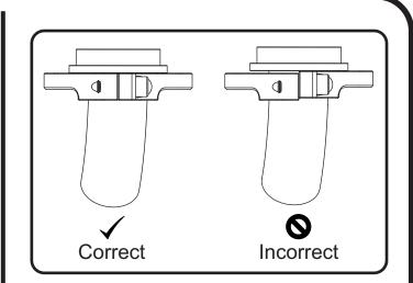
Install 13170-ADR-R1/2 rear header flange (No. 4,5) onto rear header leg using M8X25 bolts (No. 6).
