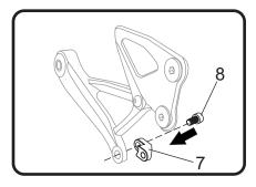
2. Align (No. 7) 13141-RMBKT, muffler bracket adapter to the backside of the right footpeg bracket. Secure using the stock bolt.
