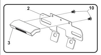
Install (No. 2) 12200-FEBKT, license plate bracket onto (No. 1) 13700-FEBKT, fender eliminator bracket using (No. 9) M6X10BHS, 6mm button head screw.
