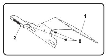
2. Secure (No. 1) *13320-FEBKT,* fender eliminator bracket to frame using (No. 6) M6X16BHS, bolts and the stock nuts.
