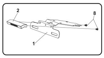
2. Install (No. 1) *11100-FEBKT*, fender eliminator bracket using (No. 7) *M6X14BHS*, 6mm button head screws. Route wires through hole in the bracket and beneath the passenger seat.
